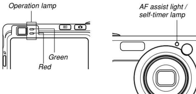
\* There are three lamp flash patterns. Pattern 1 flashes once per second, Pattern 2 flashes twice per second, and Pattern 3 flashes four times per second. The table below explains what each flash pattern indicates.
